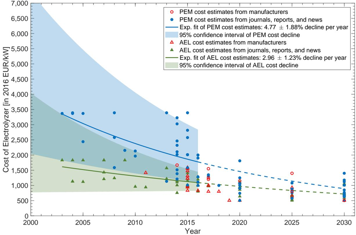
Figure 2: **Cost of electrolyzer technologies for Power-to-Gas application.** Data are from multiple sources for Alkaline Electrolysis (AEL) and Polymer Electrolyte Membrane (PEM) electrolysis.
