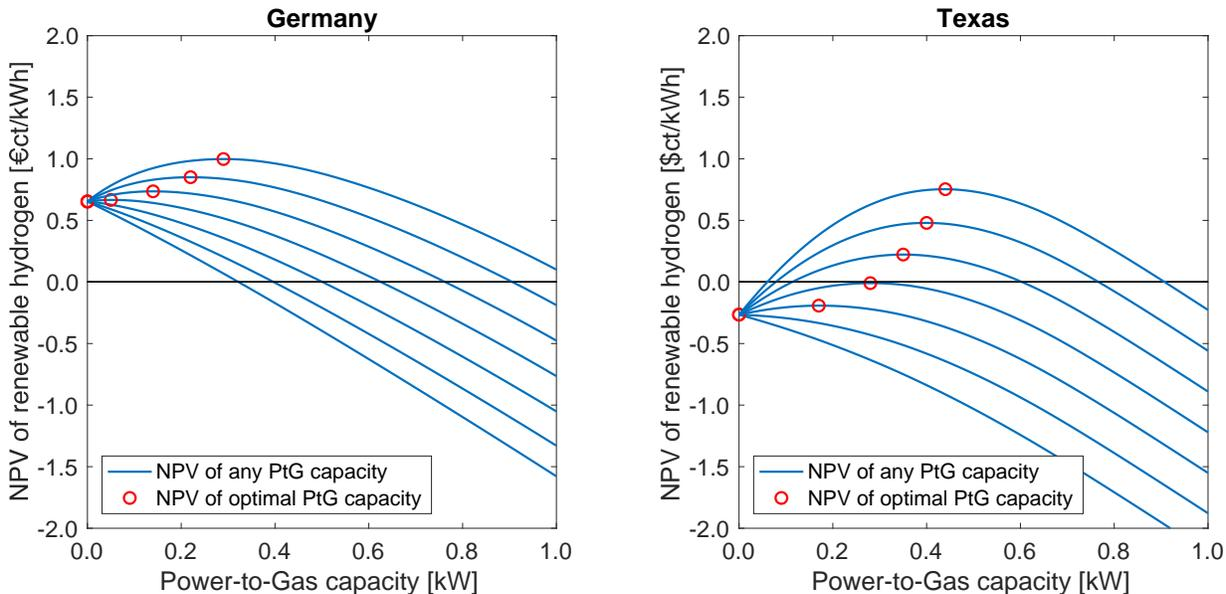
Figure 1: **Optimal Power-to-Gas capacity size and corresponding hourly profit margin.** Given a normalized wind energy capacity of 1.0 kW, the figure shows the optimized PtG capacity for alternative hydrogen prices ranging from 2.0 to 5.0 €/\$/ per kg (blue lines). The red circles mark the optimal PtG capacity size for alternative hydrogen price. Circles at 0.0 kW reflect that no PtG capacity should be installed.
